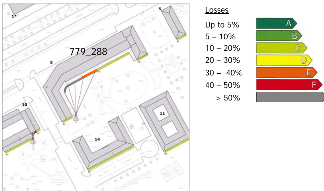
Figure 4. Passive Solar potential results: detail of an individual building assessment
